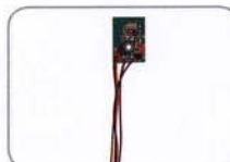
433MHz-TX Ultra-small 433MHz replacement transmitter
